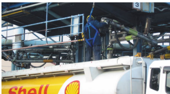
Full harness equipment has been introduced at all group refineries and depot loading areas.
