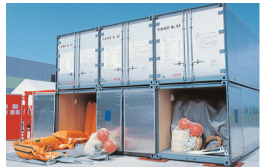
#4 stocking point for oil pollution fighting equipment/materials (at Showa Shell's Niigata Petroleum Product Import Terminal).
