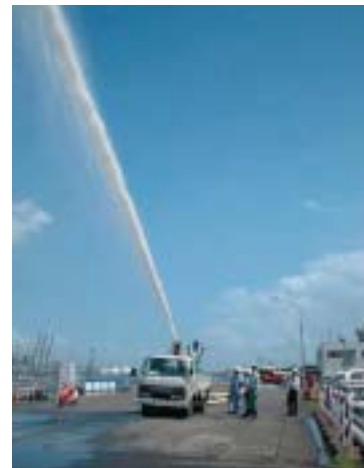
A stream from a Large-capacity Firefighting System
