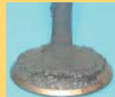
Intake valve after 16,000 km using regular gasoline
