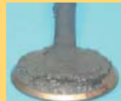
Intake valve after 16,000 km using regular gasoline
